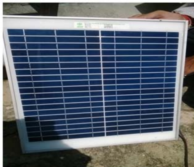
Fig.8- solar panel 20 watt
