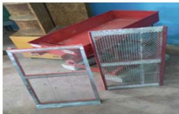
Figure 5: First and Second Layer Screens (Perforated and Screen Mesh)
