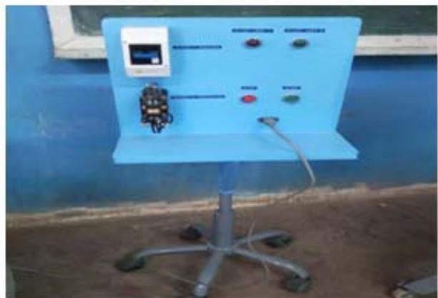
Figure 6: The Detachable Control Board
