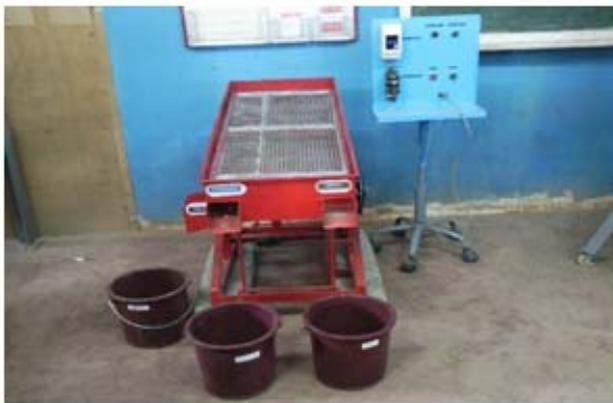
Figure 3: The Completed Remote Controlled Sand and Gravel Sorter Machine
