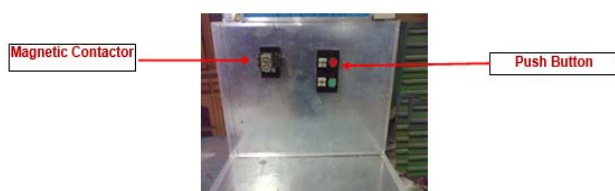
Figure 9. Metallic Wiring Board of the Trainer
