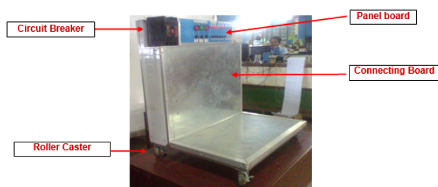
Figure 8: Completed Outcomes-Based Trainer for Tabletop Industrial Motor Control utilizing Variable Frequency Drive and Programmable Logic Controller
