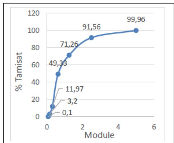
**Figure 2:** Granulometry curve of the sand used
