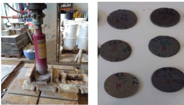
**b<sub>2</sub>)** cylindrical specimens of Ø60
