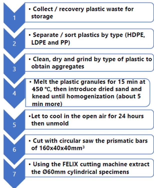
Figure 5: Methodology for manufacturing test specimens
