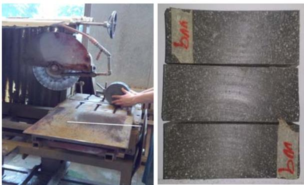
**b<sub>1</sub>)** Prismatic specimens of 160x40x40 mm<sup>3</sup>
