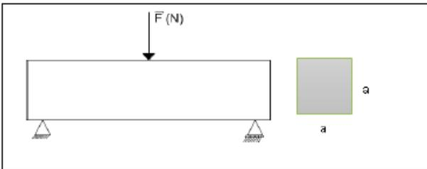
Figure 6: Geometry of the cross-section of the specimen for three-point bending test
