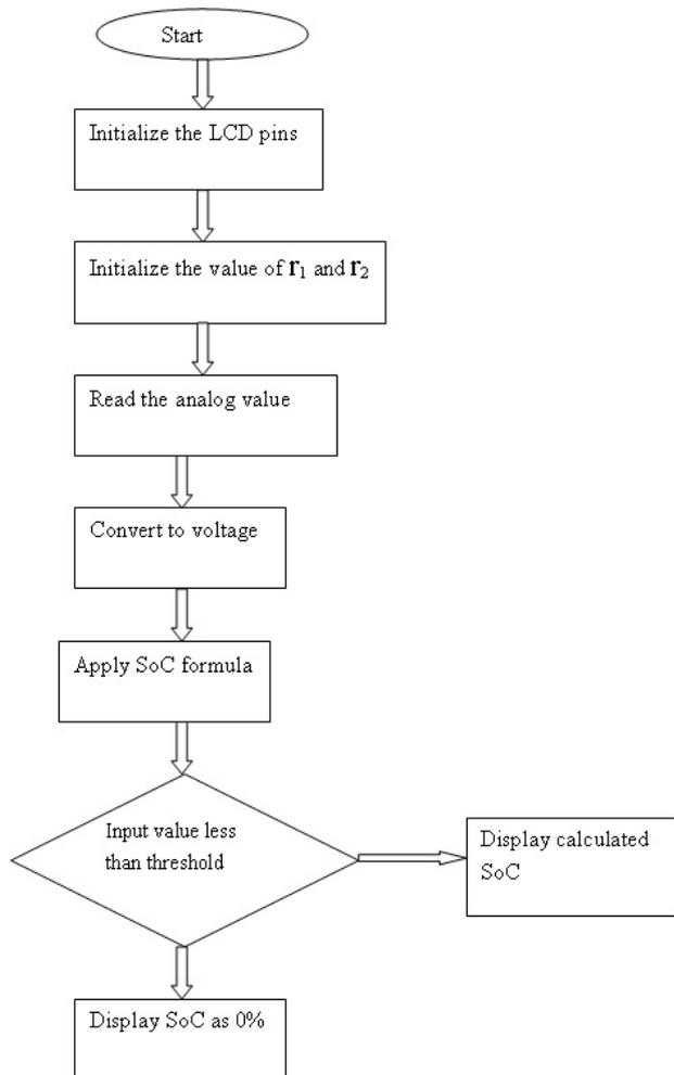
The voltage of the battery is found by mathematical calculations, which is made in arduino programming. Initially the resistor value is included and then the LCD pins are initialized. Now the analog value is converted to voltage then it is substituted in the voltage division formula. Thus the input battery voltage is found.
