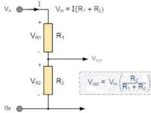
Fig 2: Voltage divider circuit
