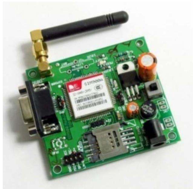
FIGURE 7: GSM MODEM (SIM900)
