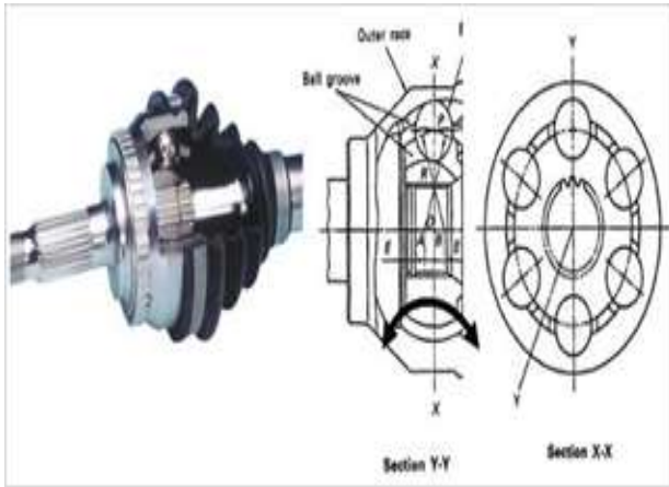
Figure-5: Typical Tripod Joint construction
