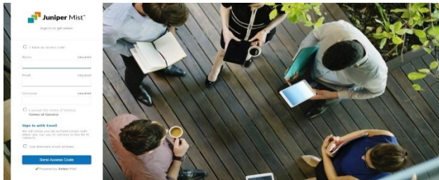
Fig. 2. Captive Portal Authentication Page for Guest Wireless Network Access using Juniper Mist Cloud.
