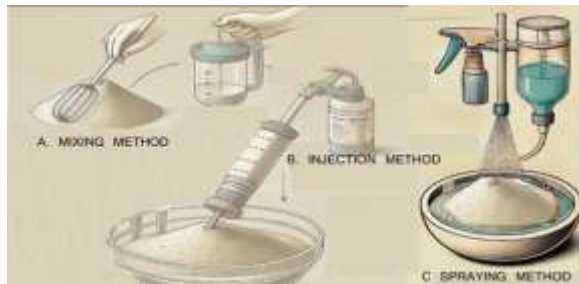
Plate I: schematic diagram for Modes of treatments considered: (a) mixing method (b) grouting method (c) spraying method]
