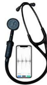
FIG. 6. Digital stethoscope and the recording app.
