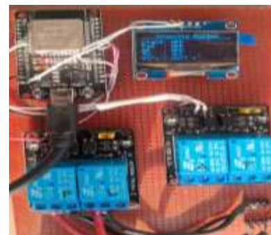
Figure 5.2: ESP32 Controller with OLED Display for System Status Monitoring
