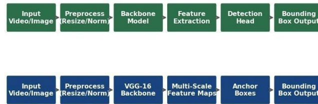
YOLOv8: Fig. 7. Syste architecture of YOLOv8 and SSD-based pothole detection system.
