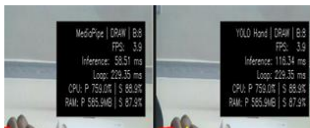
Fig. 2. Live HUD panels showing per-model FPS, inference latency, CPU%, and RAM for MediaPipe (left) and YOLOv11-Pose (right) simultaneously
