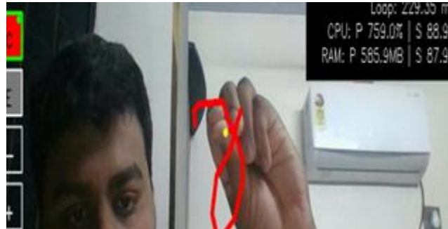
Fig. 3. Air-drawn stroke on the Virtual Canvas. Pinch gesture activates the brush; EMA smoothing ensures fluid stroke output.
