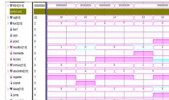
Fig. 5. Output of single cycle processor(Control Unit)
