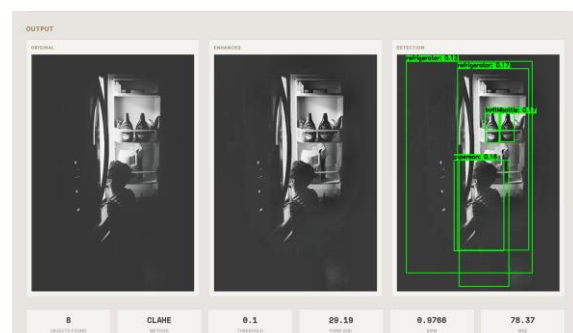
Figure 14(b): Output image after enhancement along with YOLOv8 detection.
