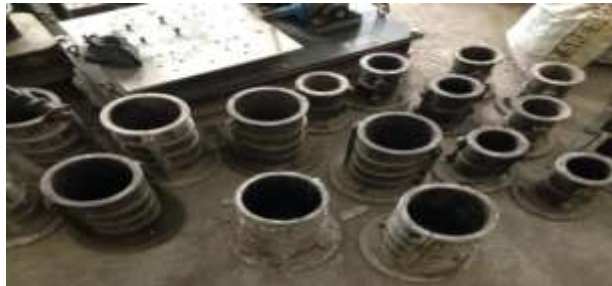
Fig. 2. Representative specimen preparation and moulding arrangement.
