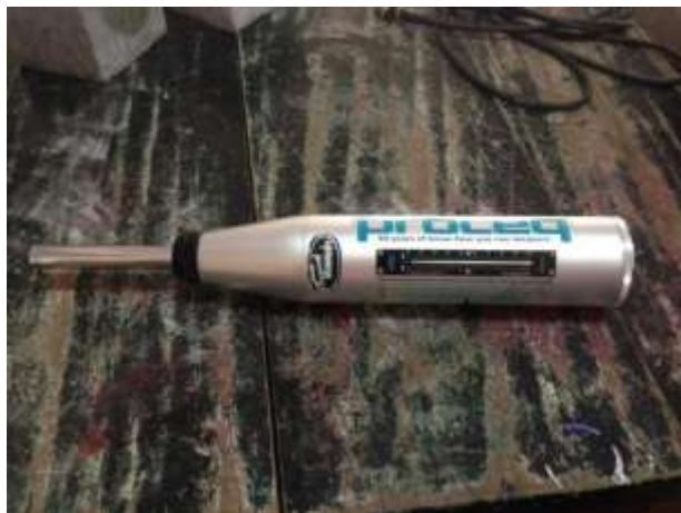
Fig. 3. Rebound hammer used for non-destructive testing.
