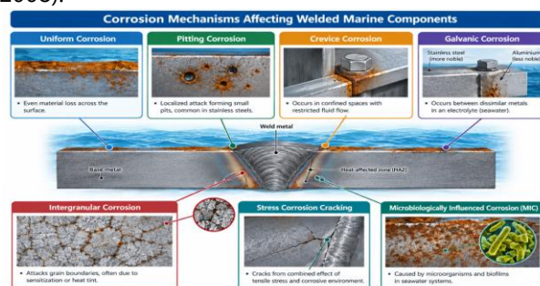
Figure 3: Major Corrosion Mechanisms Affecting Welded Marine Components in Seawater Environments
