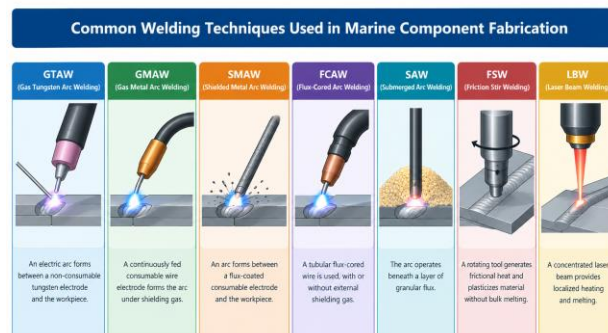
Figure 2: Common Welding Techniques Used in Marine Component Fabrication.
