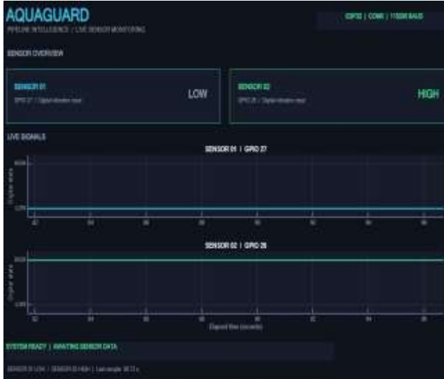
Fig. 3. AQUAGUARD MATLAB dashboard captured with the valve closed. Sensor 01 (GPIO 27) reads LOW and Sensor 02 (GPIO 26) reads HIGH; the last sample is at 96.72
