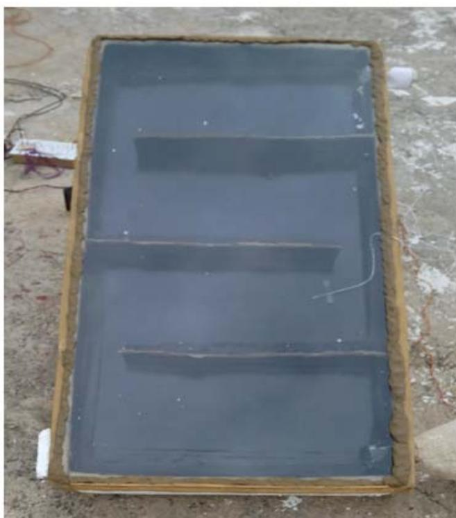
**Figure 2:** Simple single pass solar air heater with fins
