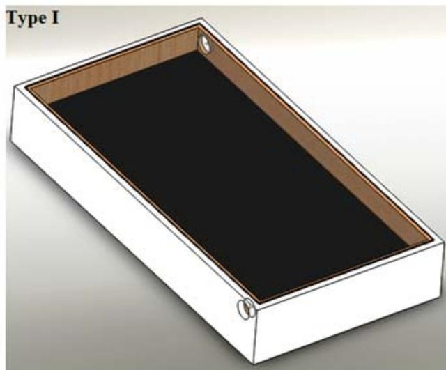
**Figure 1:** Simple single pass solar air heater without fins
