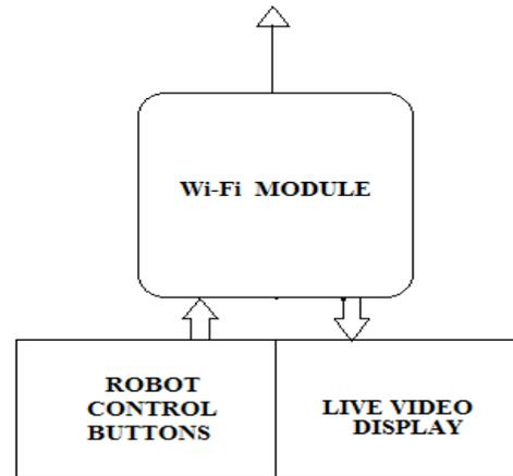
**Figure 3:** Display and control unit block diagram
