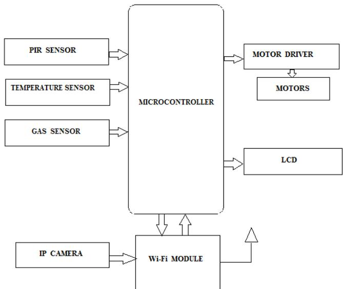
**Figure 2:** Vehicle Circuitry Block Diagram
