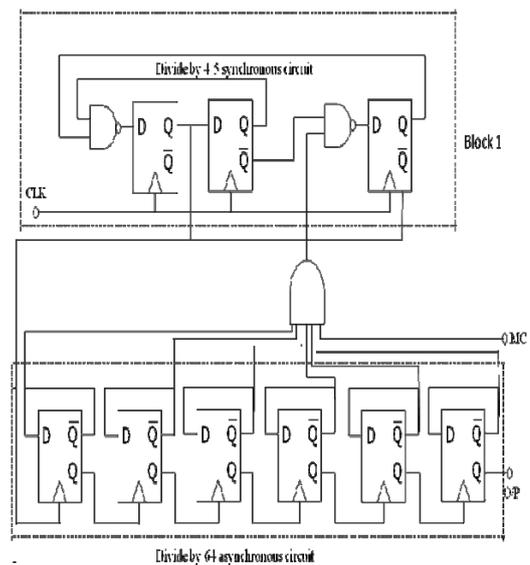
Figure 3: Functional Diagram of Dual Modulus Prescaler
