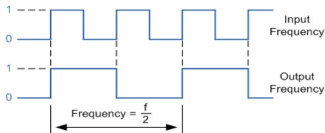
Figure 4: Output of D flip flop as Divider
