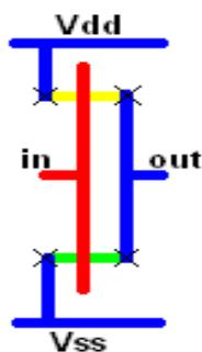
Figure 3.6: Stick Diagram of Inverter
