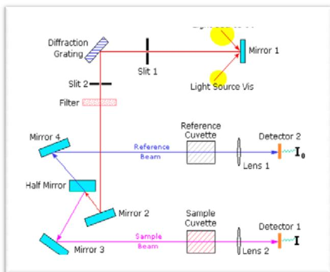
Figure 1: flow diagram uv absorption spectroscopy
