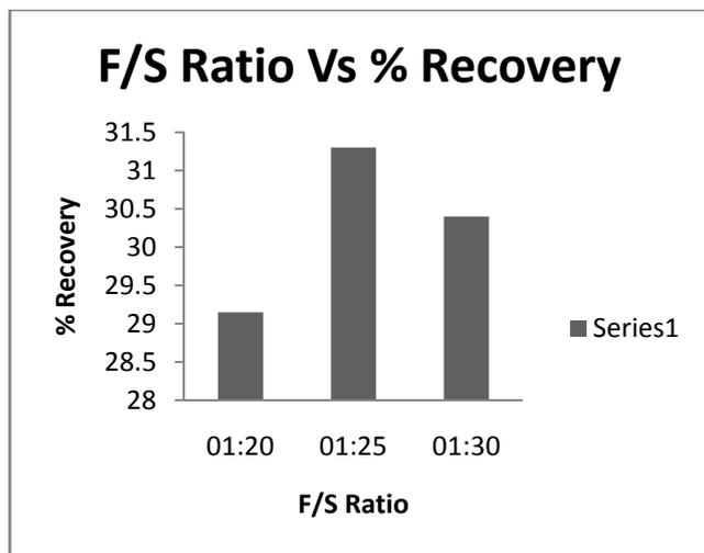
Above plot shows that maximum recovery is obtained at 1:25 ratio. The effect of solvent concentration to achieve maximum degree of tannin extraction was studied by varying the solvent concentration between 20ml to 30 ml and it was found that the optimum solvent concentration for maximum tannin extraction is 30 ml.
