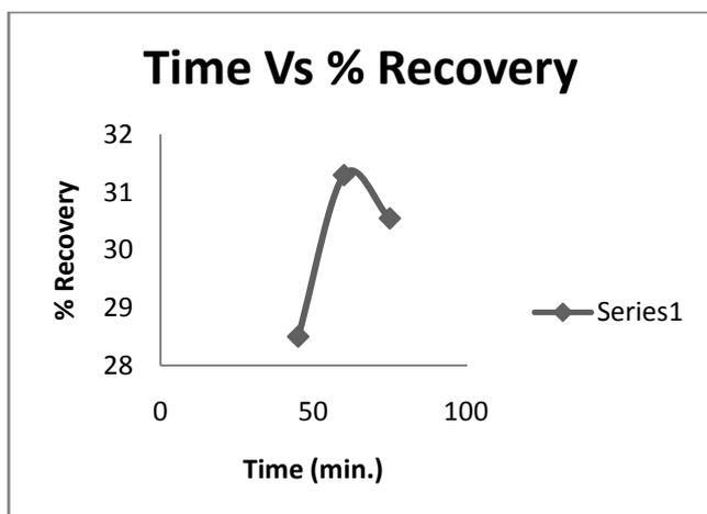
Plot shows that maximum recovery is obtained at 60 minutes of contact time. The effect of time to achieve maximum degree of tannin extraction was studied by varying the time period between 45 min to 75 min and it was found that the optimum time period for maximum tannin extraction is 60 minutes.
