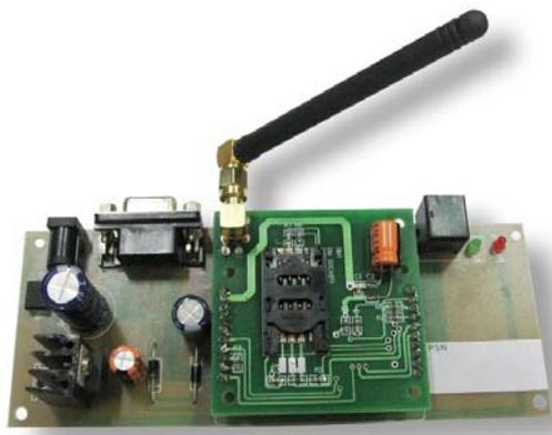
Figure 4: GSM module
