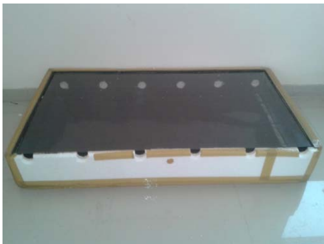
Figure 5: solar dryer with thermocol insulation
