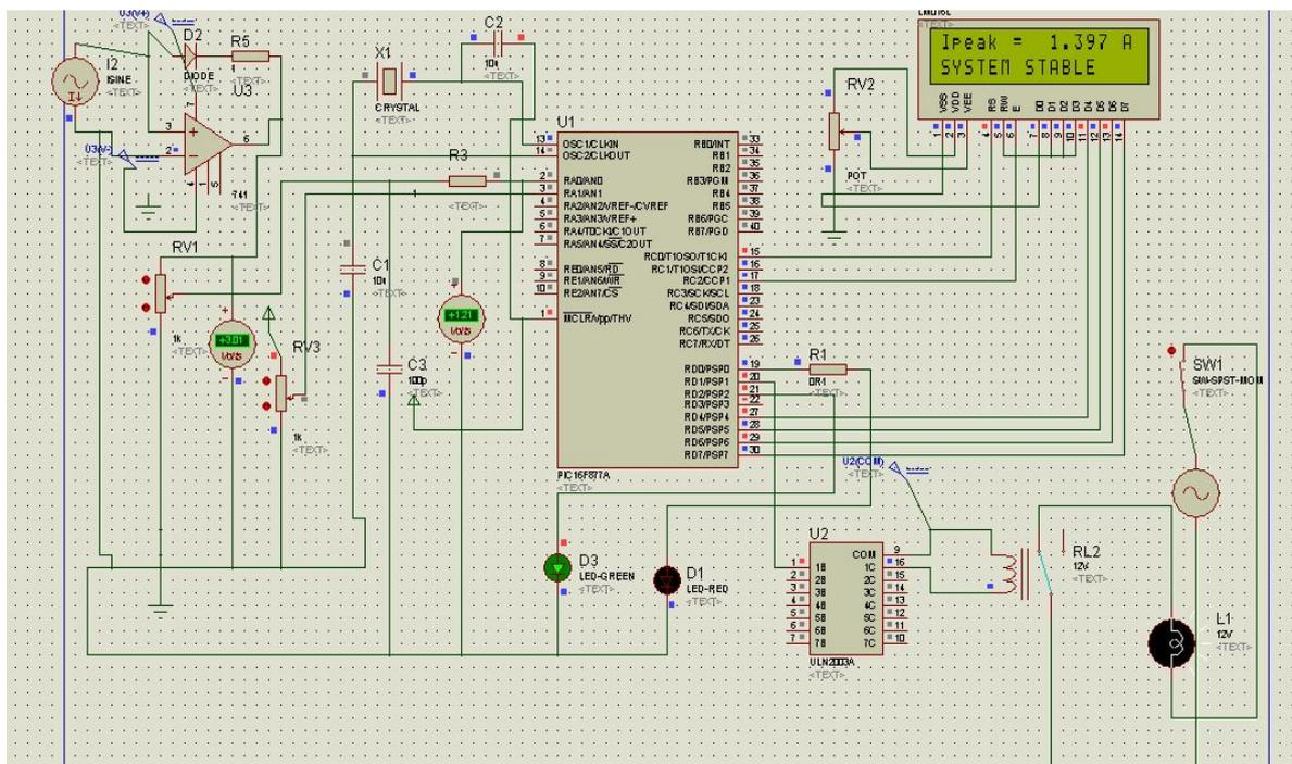
Figure 7: Proteus schematic of Microcontroller based Overcurrent relay showing the Normal Operation
