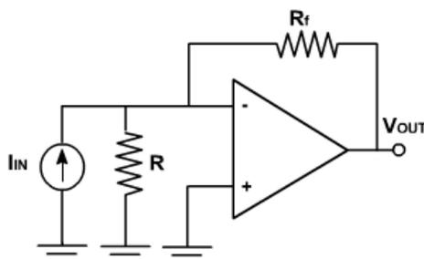
Fig 2: I to V Converter
