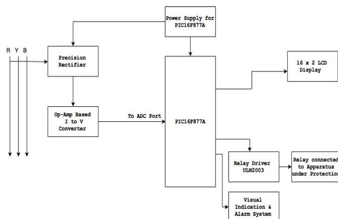
Figure 1: Block diagram of the simulation circuit using microcontroller relay
