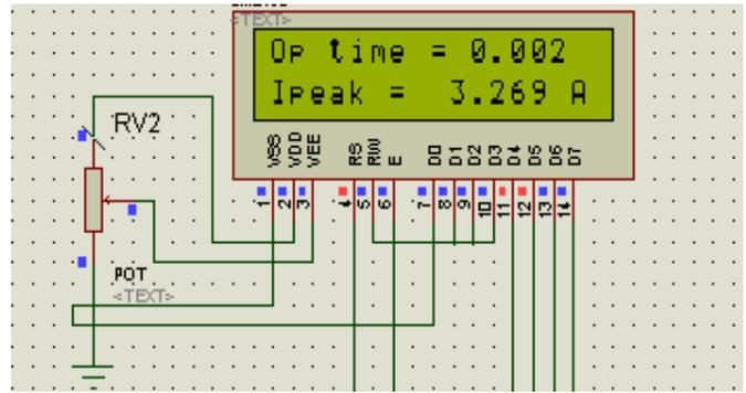
Figure 5: Proteus schematic of Microcontroller based relay showing the tripping status with the current value
