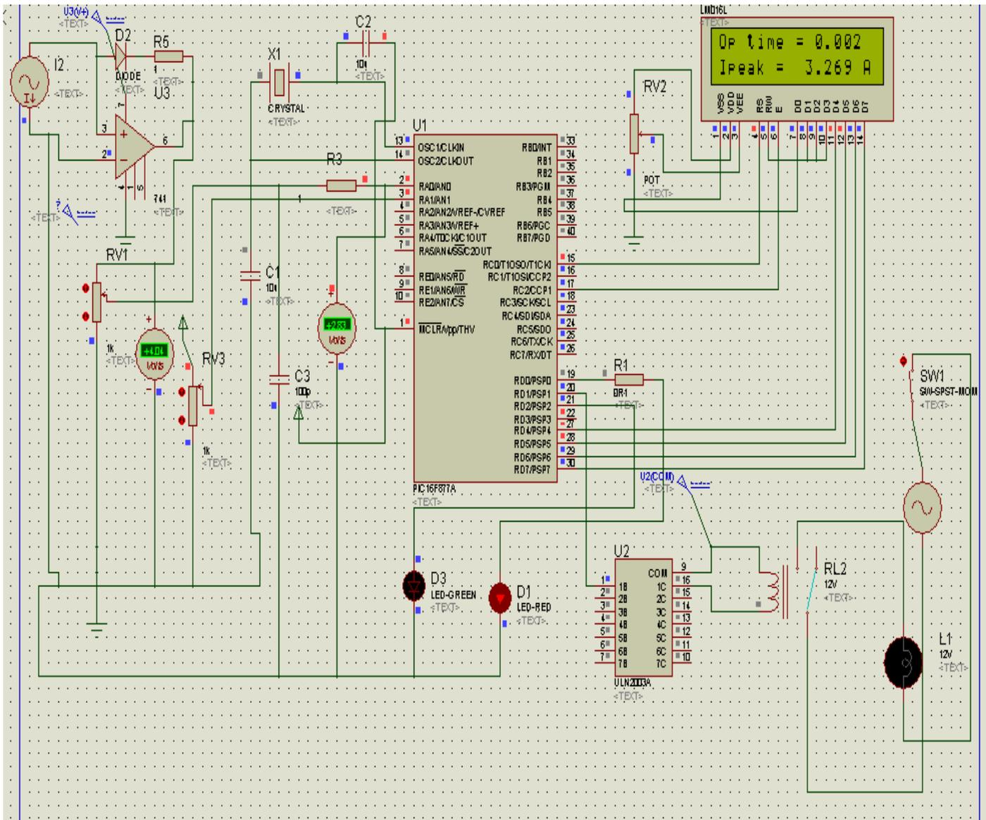
Figure 3: Proteus schematic showing the operating time and the current at the time of tripping
