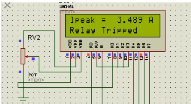
Figure 4: LCD indicating status of relay (tripping state)
