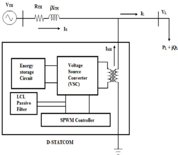
Figure 2.1.1: Schematic diagram of a D-STATCOM
