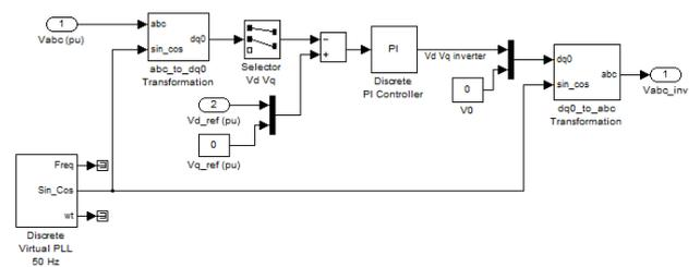
Fig.2.1.3: Block Diagram of Controller System
