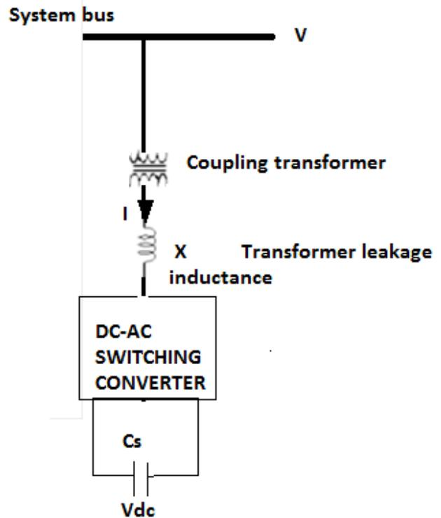
Figure 2.1.2: Operation mode of Voltage Source Converter
