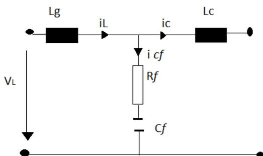
Figure 2.1.4: LCL Passive Filter
