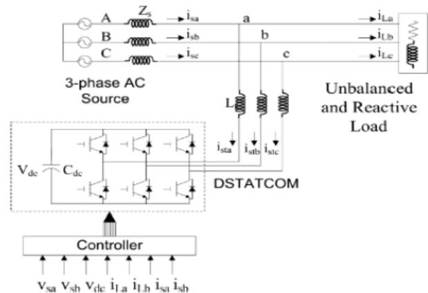
Figure 1.1: Basic Circuit Diagram of the DSTATCOM System.
