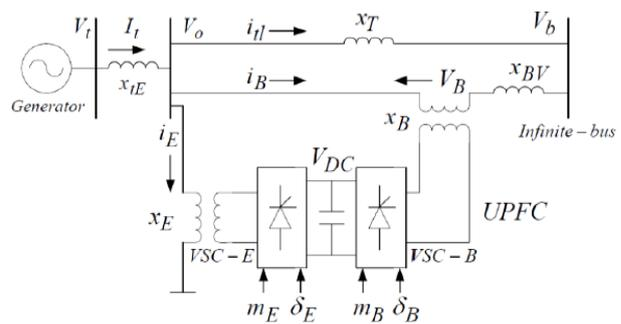
Fig.3 Power system connected to infinite bus with UPFC
