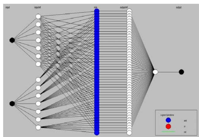
Fig.4. structure of adaptive neuro-fuzzy controller
