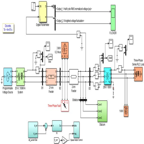
Fig.5. Simulation Model for SVPWM Controller
