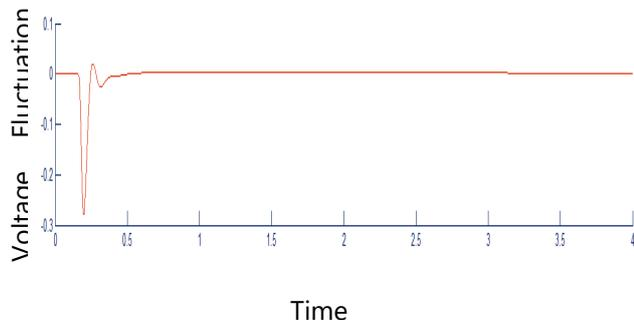
Fig.7. Fluctuation voltage without fault (SVPWM STATCOM)
