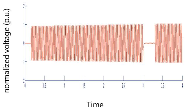
Fig. 8. Half cycle normalized voltage with fault (SVPWM STATCOM)
