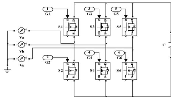
Fig.3. Simulation Model of Voltage Source Converter
