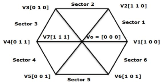
Fig.4. Principle of Space Vector used in VSC
