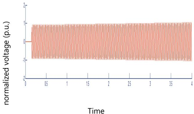
Fig. 6 Half cycle normalized voltage without fault (SVPWM STATCOM)
