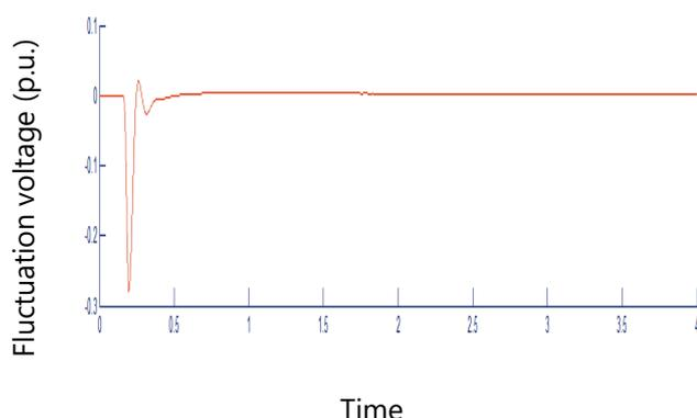
Fig. 9. Fluctuation voltage with fault (SVPWM STATCOM)
