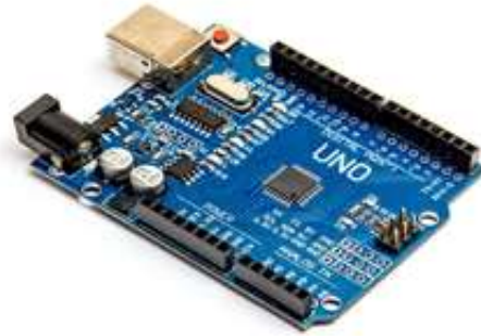
Fig-4: Arduino Uno used as a Primary Micro Controller
