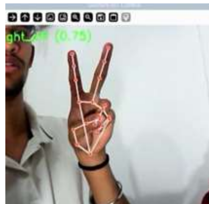
Fig. 2. Gesture-Based Activation of Light (ON State)
