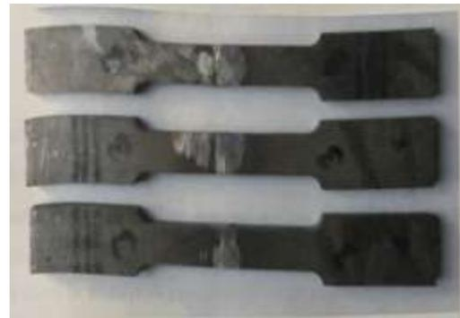
Figure 7: Transverse tensile test specimens
