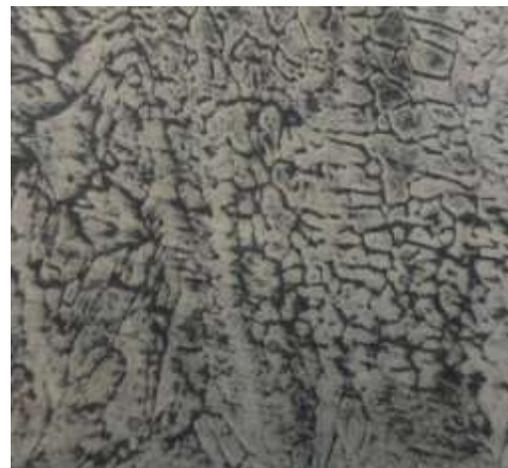
Figure 15: Micrograph of Joint 1 (groove angle  $45^{\circ}$ )
