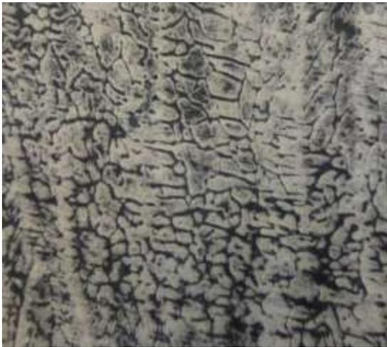
Figure 16: Micrograph of joint 2 (groove angle 60°)
