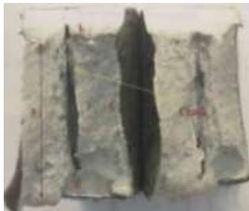
Figure 6: Fractured view of Charpy V- notch (Joint-3, Groove angle 75°)
