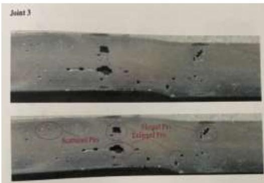
Figure 10: View of joint-3 after Pitting Corrosion
