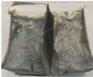
Figure 5: Fractured view of Charpy V-Notch (Joint-2, Groove angle 60°)
