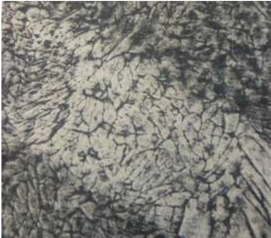
Figure 17: Micrograph of Joint 3 (groove angle 75°)
