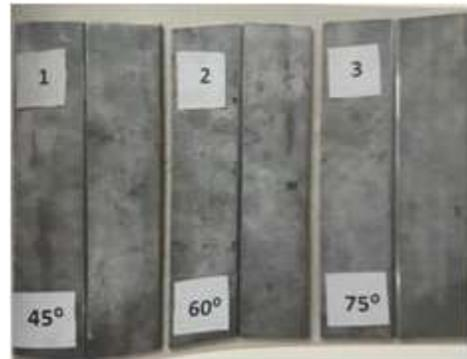
Figure 2: Top View of Sample with different groove angle
