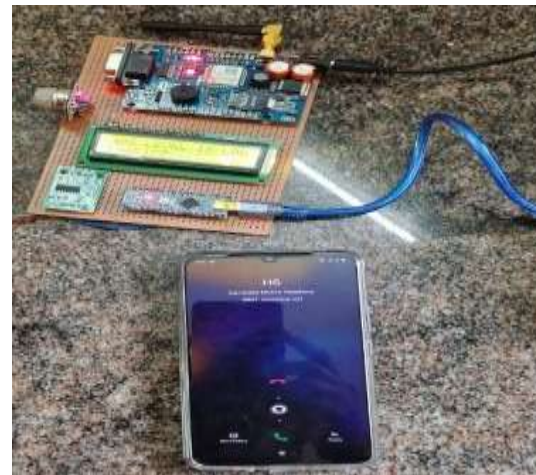
Fig 3: Call to user when gas level is low
