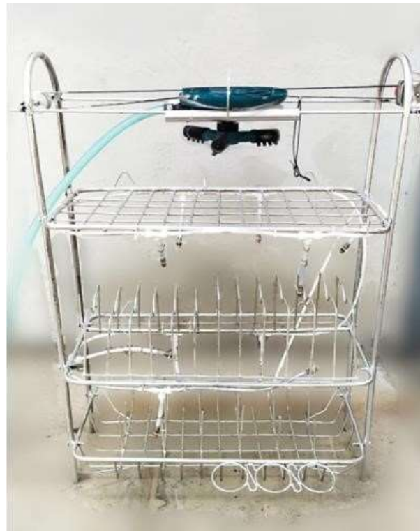
Figure 8: Dishwasher Stand (Cover removed)
