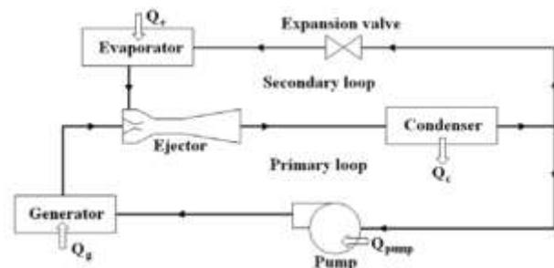
Figure 1: A basic ejector refrigeration cycle
