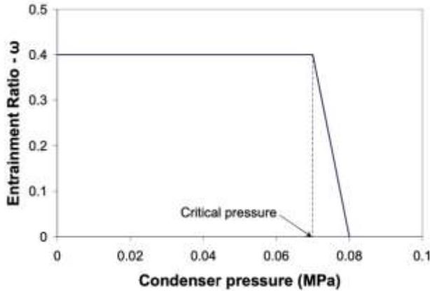
Figure 2: Ejector characteristics
