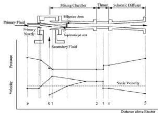
Figure 3: Typical ejector geometry, pressure and velocity profiles along ejector length [1]
