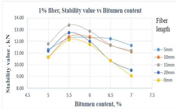
Figure.10 The fluctuation of stability values concerning different bitumen content in 1% fiber content at different fiber length
