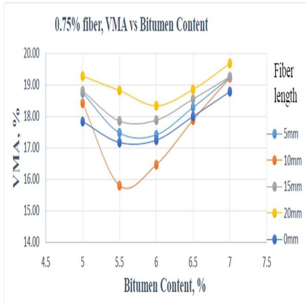
Figure.25 The fluctuation of % VMA concerning different bitumen content in 0.75% fiber content at different fiber length
