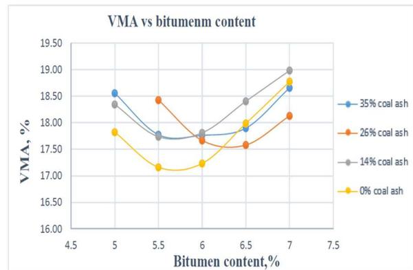
Figure 5. The fluctuation of VMA concerning different levels of bitumen content at varying coal ash concentrations
