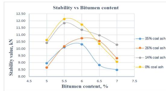
Figure 1 The fluctuation of stability values concerning different levels of bitumen content at varying coal ash concentrations
