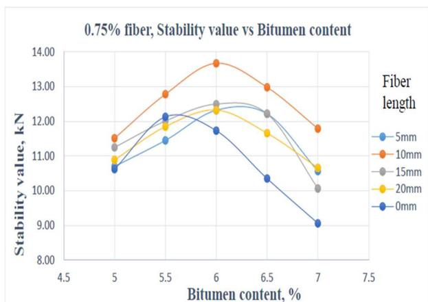
Figure.9 The fluctuation of stability values concerning different bitumen content in 0.75% fiber content at different fiber length
