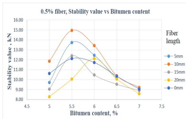
Figure.8 The fluctuation of stability values concerning different bitumen content in 0.5% fiber content at different fiber length
