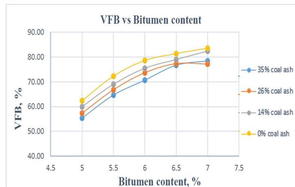
Figure 6 The fluctuation of VFB concerning different levels of bitumen content at varying coal ash concentrations
