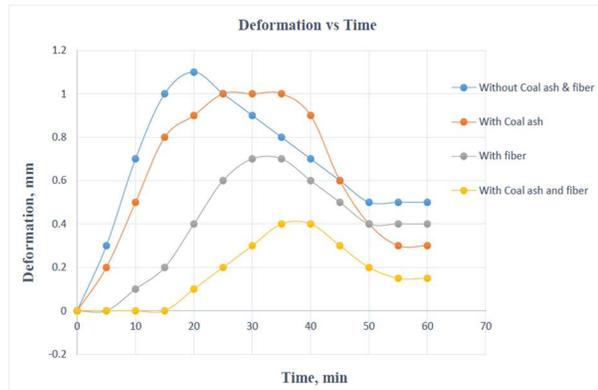
Figure 33 Changes in deformation values at 40°C, over time for the DBM sample.
