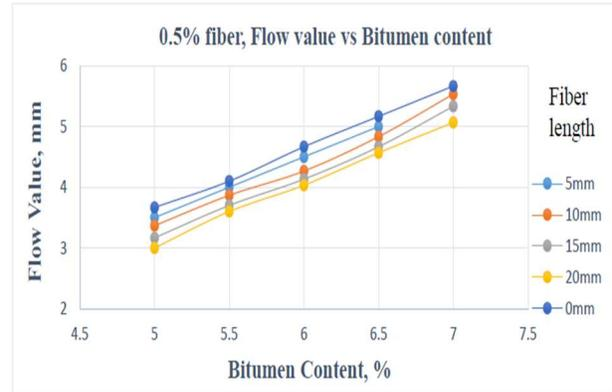
Figure.12 The fluctuation of flow values concerning different bitumen content in 0.50% fiber content at different fiber length
