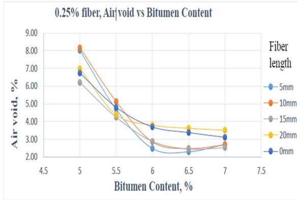
Figure.19 The fluctuation of % air void concerning different bitumen content in 0.25% fiber content at different fiber length
