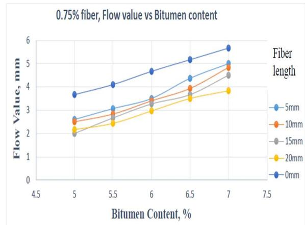
Figure.13 The fluctuation of flow values concerning different bitumen content in 0.75% fiber content at different fiber length
