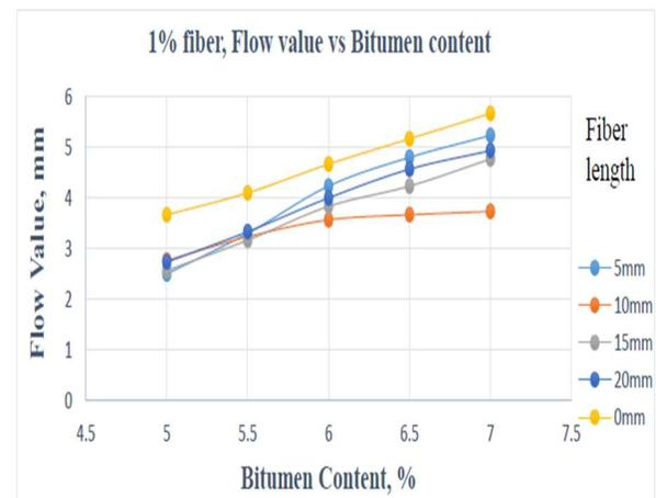
Figure.14 The fluctuation of flow values concerning different bitumen content in 1% fiber content at different fiber length
