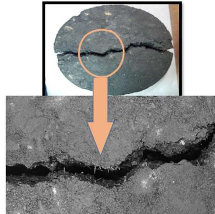
Figure.31 Sisal fiber distribution in a crisscross pattern observed at the point of tensile failure crack.
