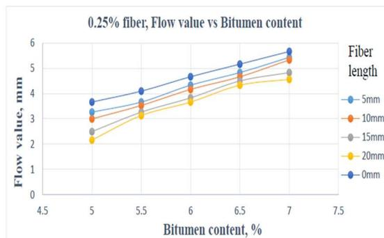
Figure.11 The fluctuation of flow values concerning different bitumen content in 0.25% fiber content at different fiber length
