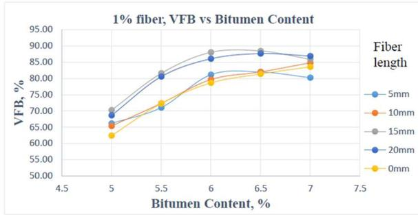
Figure.30 The fluctuation of % VFB concerning different bitumen content in 1% fiber content at different fiber length
