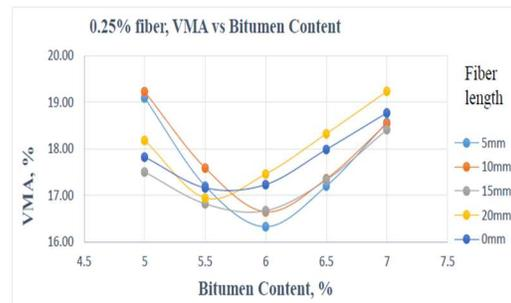
Figure.23 The fluctuation of % VMA concerning different bitumen content in 0.25% fiber content at different fiber length
