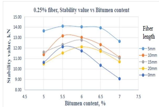
Figure.7 The fluctuation of stability values concerning different bitumen content in 0.25% fiber content at different fiber length
