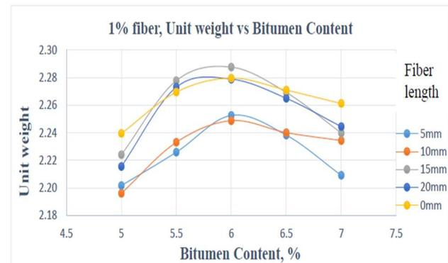
Figure.18 The fluctuation of Unit weight concerning different bitumen content in 1% fiber content at different fiber length
