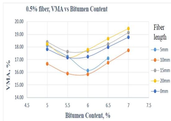
Figure.24 The fluctuation of % VMA concerning different bitumen content in 0.5% fiber content at different fiber length
