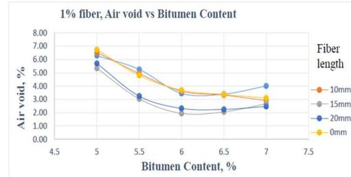
Figure.22 The fluctuation of % air void concerning different bitumen content in 1% fiber content at different fiber length
