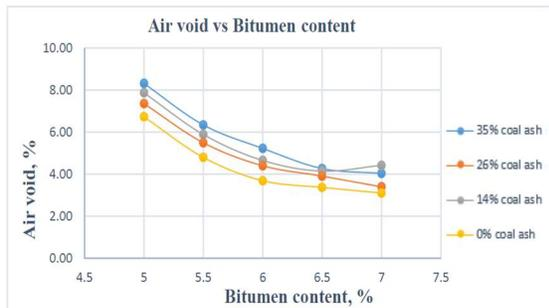
Figure 3 The fluctuation of Air Void concerning different levels of bitumen content at varying coal ash concentrations
