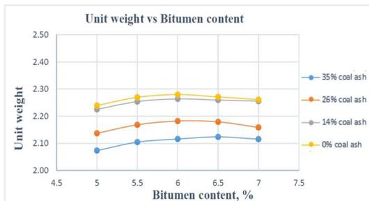
Figure .4 The fluctuation of Unit weight concerning different levels of bitumen content at varying coal ash concentrations
