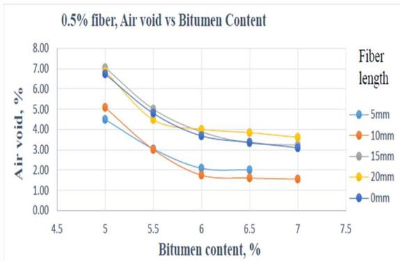
Figure.20 The fluctuation of % air void concerning different bitumen content in 0.5% fiber content at different fiber length
