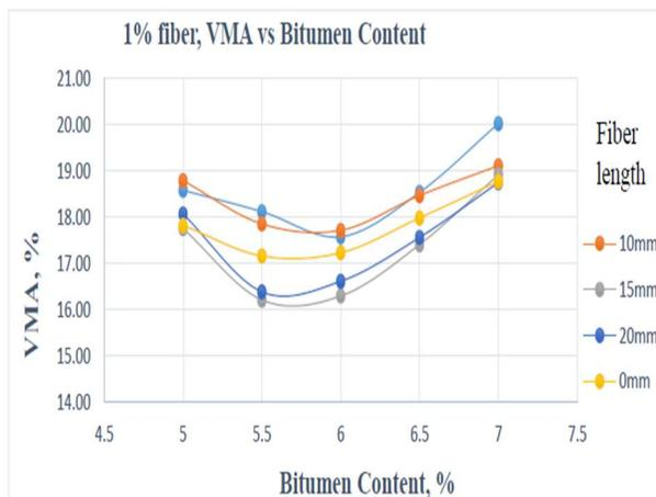
Figure.26 The fluctuation of % VMA concerning different bitumen content in 1% fiber content at different fiber length
