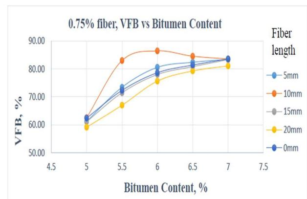
Figure.29 The fluctuation of % VFB concerning different bitumen content in 0.75% fiber content at different fiber length
