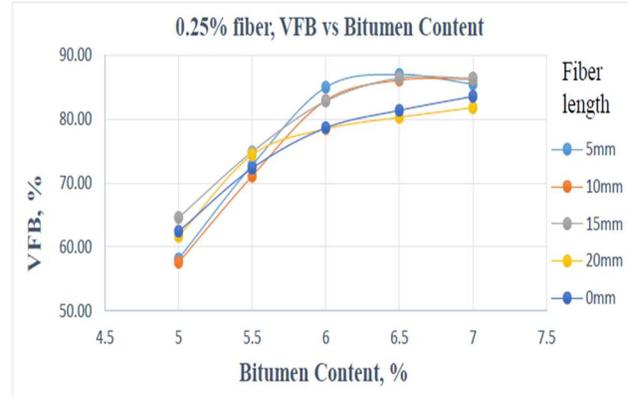
Figure.27 The fluctuation of % VFB concerning different bitumen content in 0.25% fiber content at different fiber length
