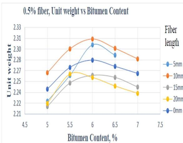
Figure.16 The fluctuation of Unit weight concerning different bitumen content in 0.5% fiber content at different fiber length
