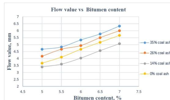
Figure 2 The fluctuation of Flow values concerning different levels of bitumen content at varying coal ash concentrations
