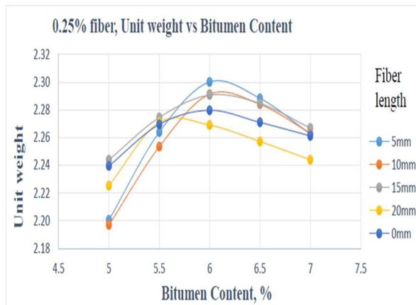
Figure.15 The fluctuation of Unit weight concerning different bitumen content in 0.25% fiber content at different fiber length
