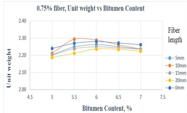
Figure.17 The fluctuation of Unit weight concerning different bitumen content in 0.75% fiber content at different fiber length
