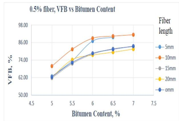
Figure.28 The fluctuation of % VFB concerning different bitumen content in 0.5% fiber content at different fiber length
