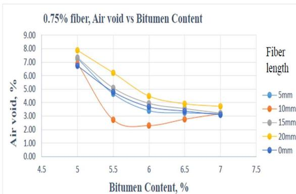
Figure.21 The fluctuation of % air void concerning different bitumen content in 0.75% fiber content at different fiber length
