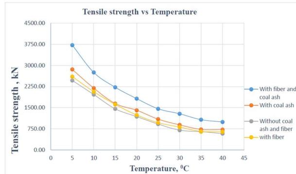
Figure.32 Graph between Tensile strength vs Temperature.
