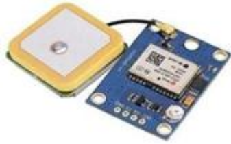
Figure 5.3: NEO-6M GPS Module
