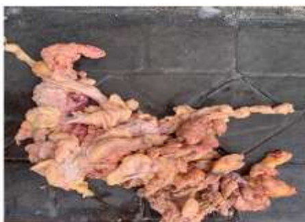
Figure 3: Raw beef tallow used for transesterification
