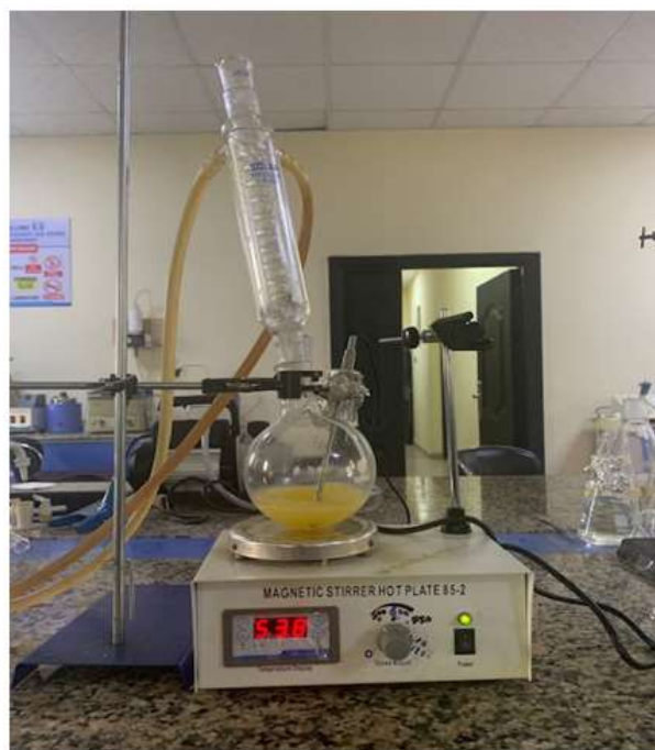
Figure 4: Reaction of beef tallow to produce biodiesel
