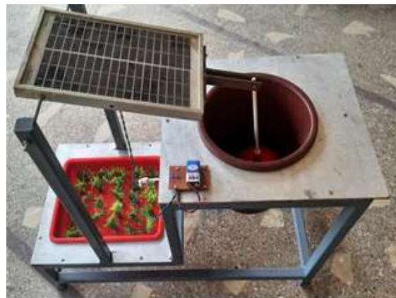
Figure 1. Mechanical Solar Tracking System
