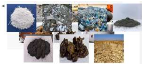
Figure 1: Materials for the development of Redone bricks: a) Lime, b) C&D Debris, c) Plastic Debris, d) Fly Ash, e) Aluminum Powder, e) Guggul, f) Agricultural Waste
