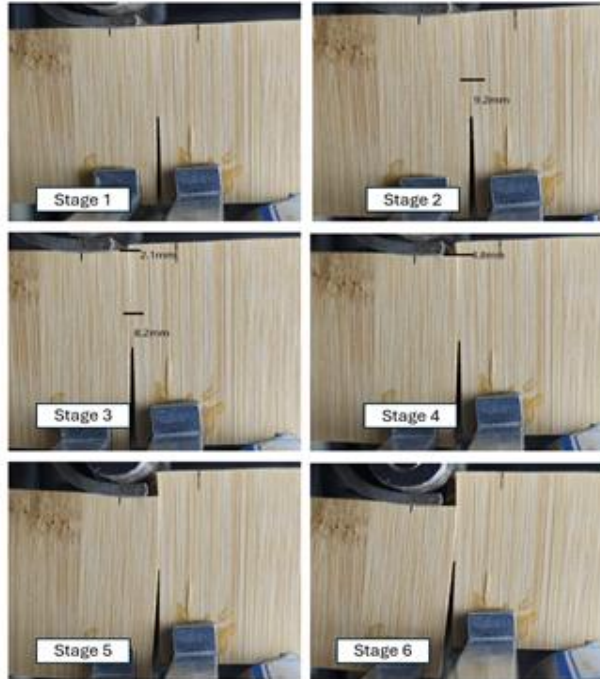
Figure 9:Fracture process for Group 5 ( (0/90)_2/0 , a/h = 0.5 )
