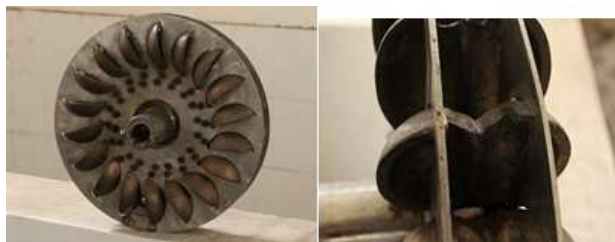
Fig. 4. Novel hooped runner with bucket arrangement between two flanges
