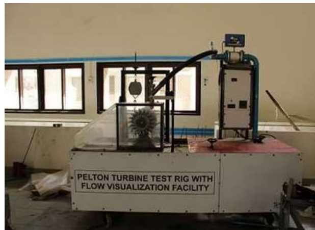
Fig. 2. Experimental setup with traditional runner
