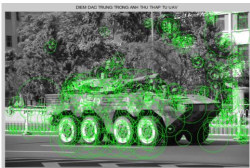
Figure 2: Feature points within the armored vehicle reference template and the UAV-acquired image.
