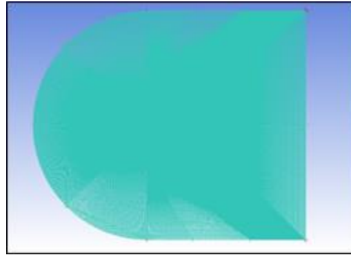
Figure 5. Structured Mesh of Wedge Convex Airfoil
