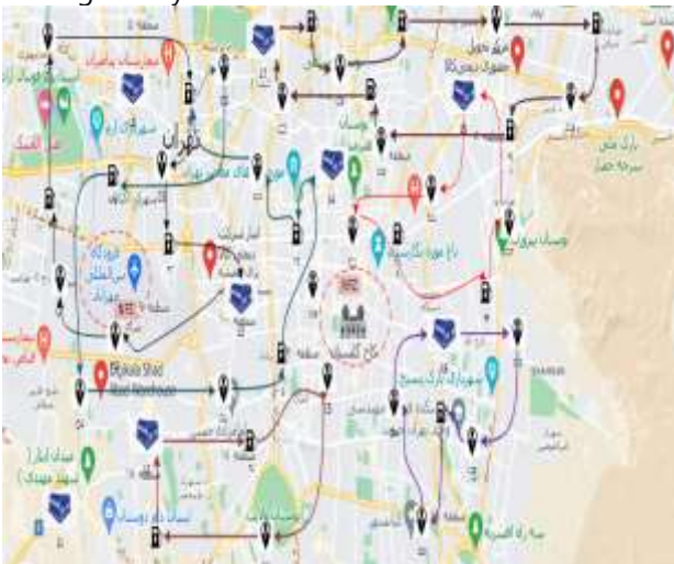
Figure 14. A sample operational flight path for a UAV (UAV 2) within the optimized Tehran network. The route originates from a central depot, services multiple customers, includes stops at intermediate charging stations, and finally returns to the base. Numbers along the path indicate the stop sequence. This route was generated while adhering to all capacity, time-window, and no-fly zone constraints of the model.
