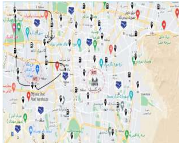
Figure 14. A sample operational flight path for a UAV (UAV 2) within the optimized Tehran network. The route originates from a central depot, services multiple customers, includes stops at intermediate charging stations, and finally returns to the base. Numbers along the path indicate the stop sequence. This route was generated while adhering to all capacity, time-window, and no-fly zone constraints of the model.
