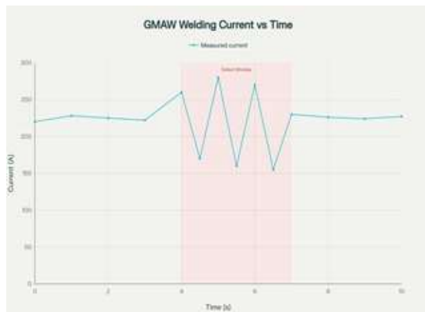
Graph 1.2: GMAW welding current signal with an unstable region associated with a defect event between 4 and 7 seconds.
