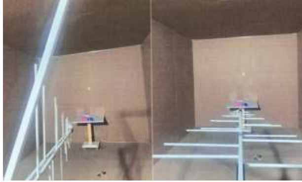
Figure 2. Radiated emission measurements of thermal pad
