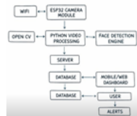
Fig.2. System Flowchart illustrating the initialization, connection handling, and recognition loop.
