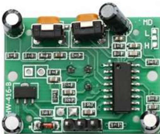
Fig 4.3 PIR motion sensor
