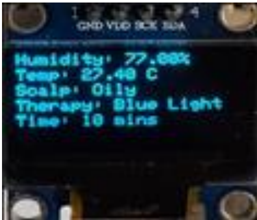
Figure 4: OLED Display Showing Scalp Condition and Therapy Recommendation with Duration
