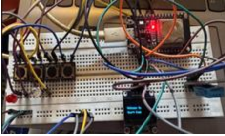
Figure 7: Complete Hardware Setup of the Smart Hair Comb Prototype
