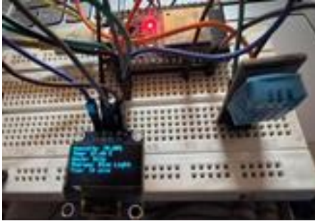
Figure 3: OLED Display Indicating Humidity, Temperature, Scalp Condition, and Therapy Mode
