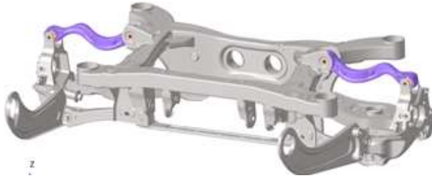
Figure 1: Typical multi-link rear suspension architecture.
